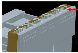
STEP 1: INSTALL RISERS (2601156) TO FLUE USING CABINET SCREWS (8090412). TWO PER FRYPOT.
